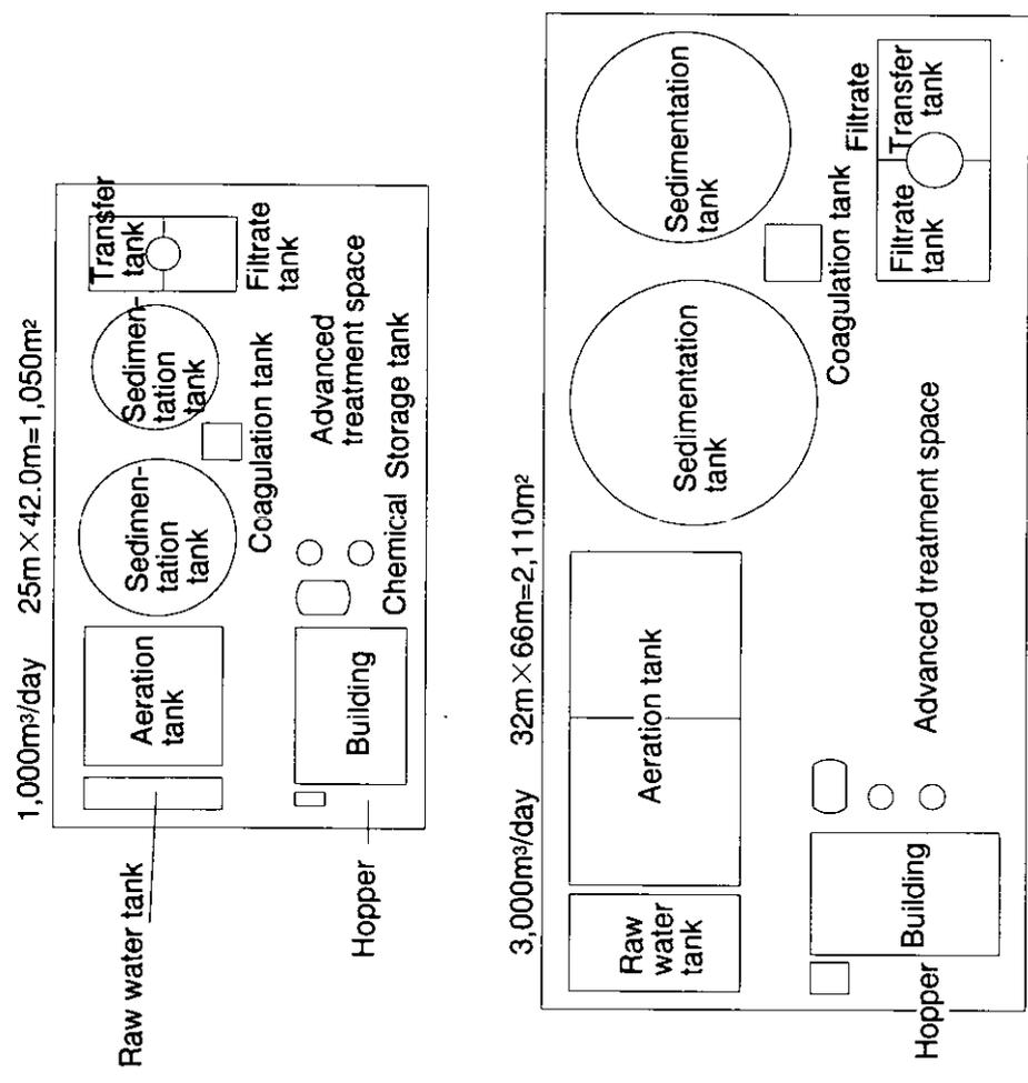
Figure-3 Treatment facility plane layout drawing
