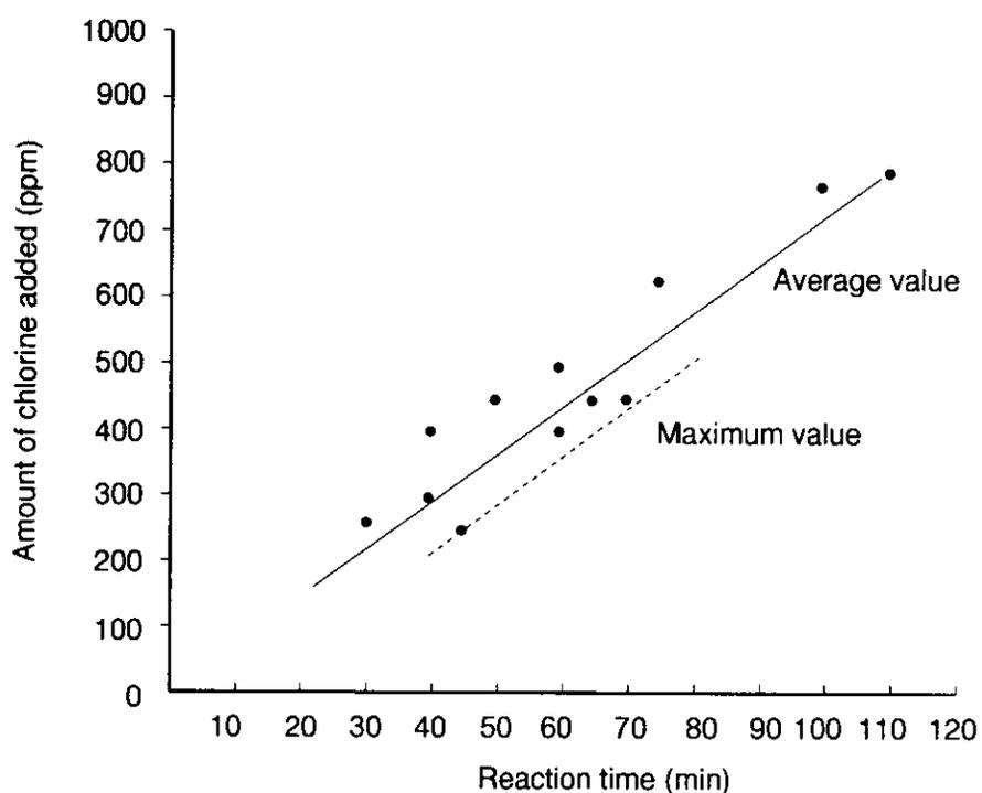
Figure-9 Relation between Amount of Added chlorine and Reaction Time in Batch Type
