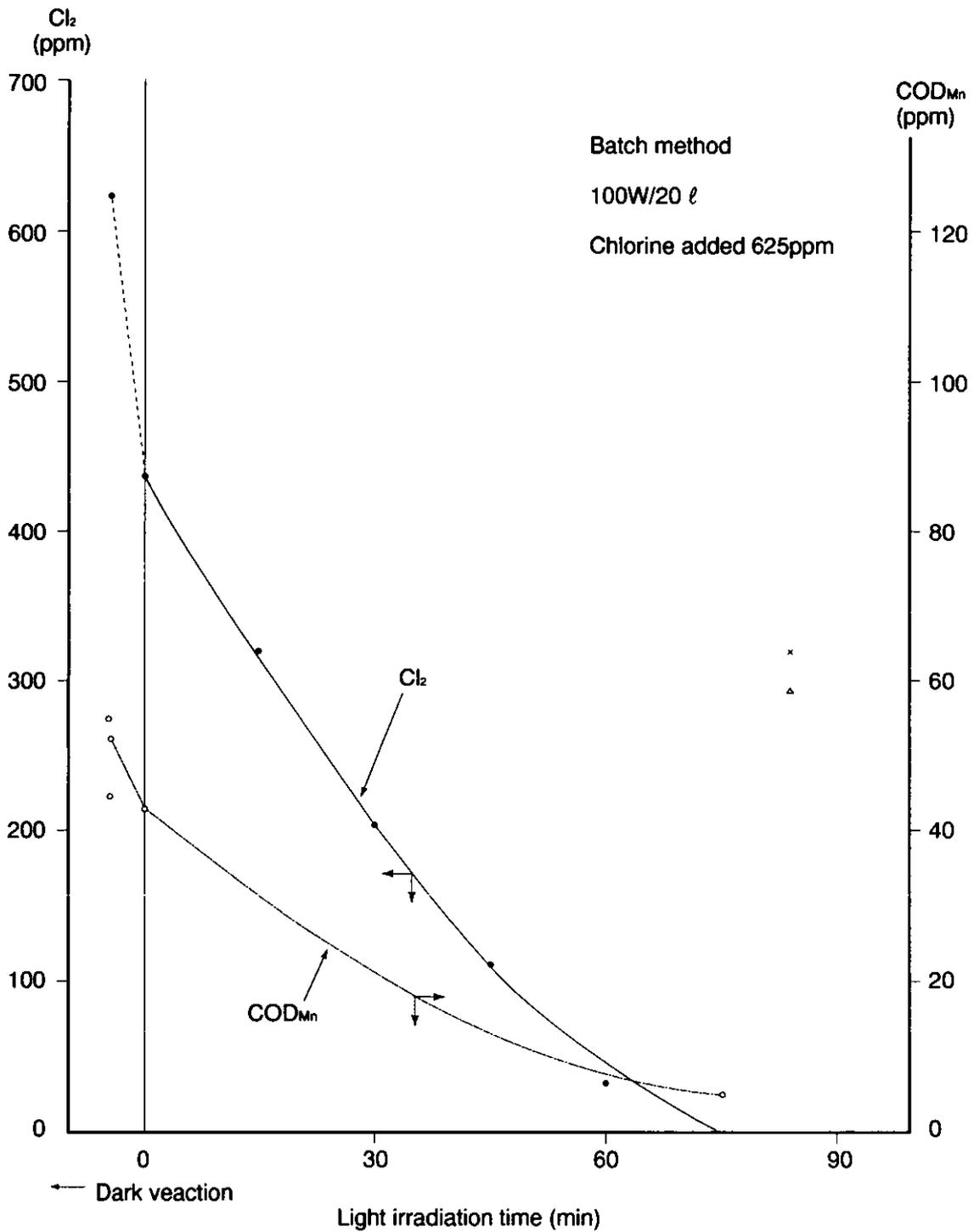
Figure-5 Batch type test result (wastewater of Oct. 28)
