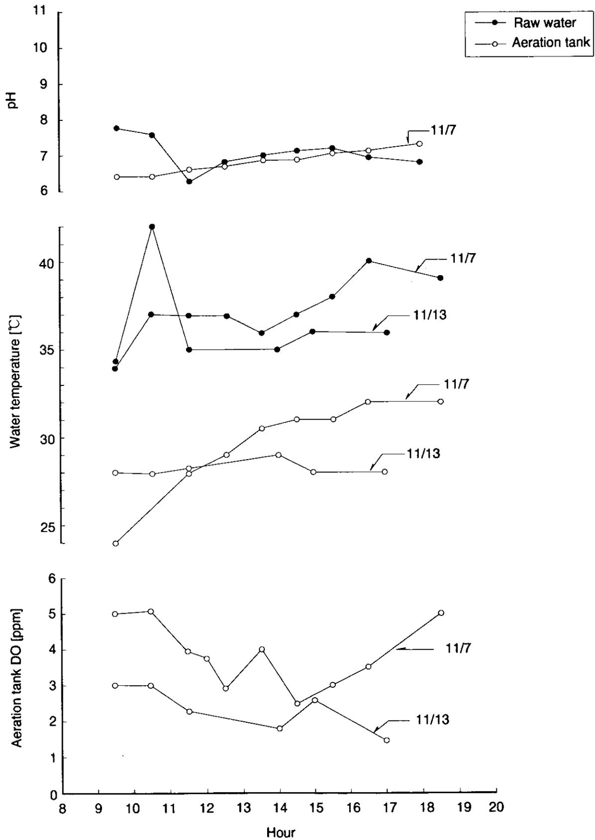
Appended figure-3 Hourly variation in aeration tank DO, water temperature and pH (RUN 2)
