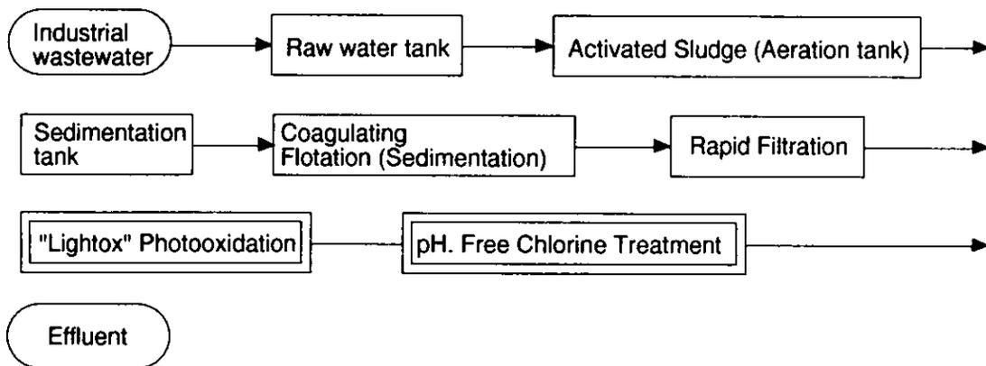
A process in a dual square corresponds to one for which the cost of equipment was calculated in Item (6).
