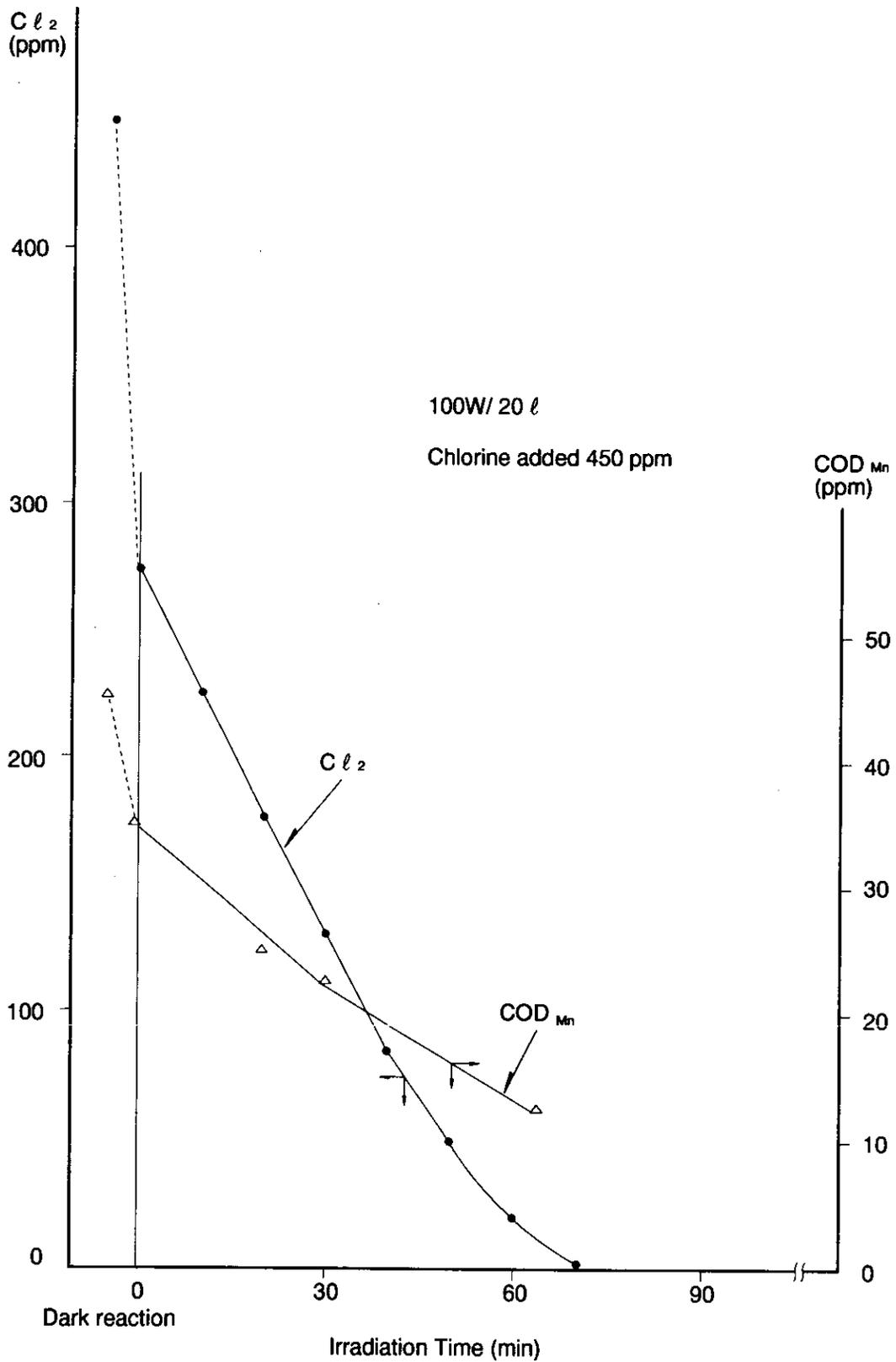
Figure-7 Batch type test result (wastewater of Nov 6)
