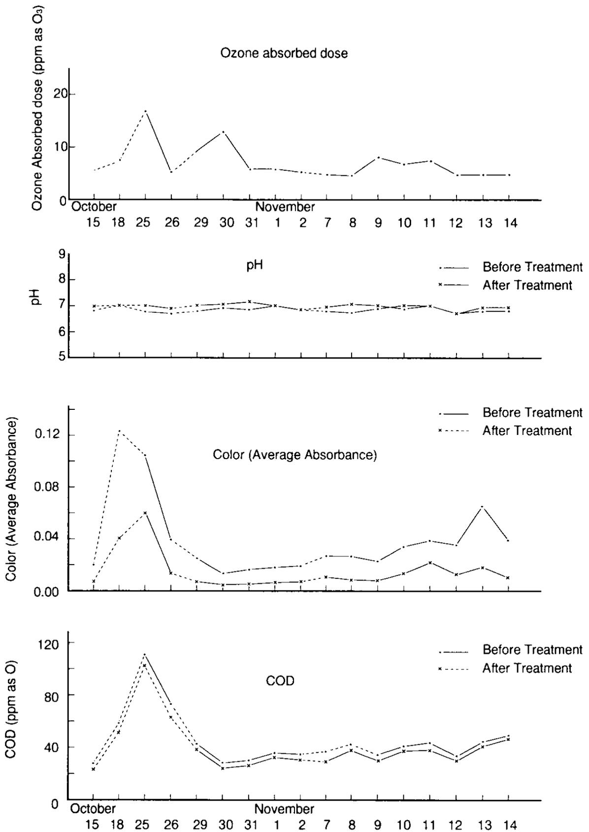
Figure-3 Result of Experiment on Oxidation by Ozone with Secondary Effluent
