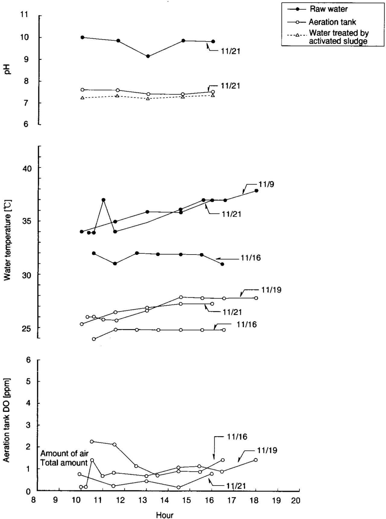
Appended figure-4 Hourly variation in aeration tank DO, water temperature and pH (RUN 3)
