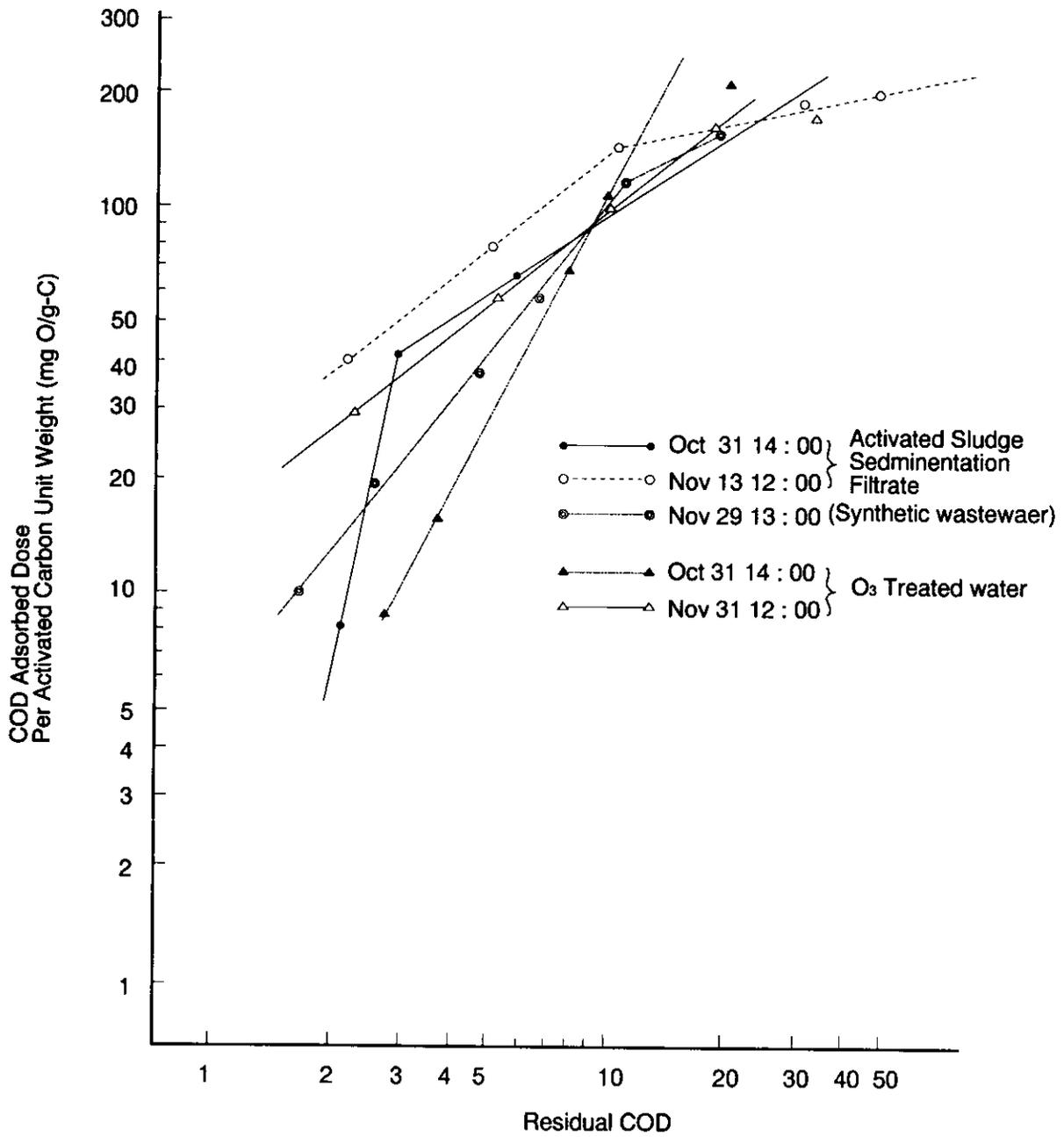
Figure 8 Activated carbon Equilibrium absorption diagram for Secondary Effluent and Secondary Effluent Treated by Ozone
