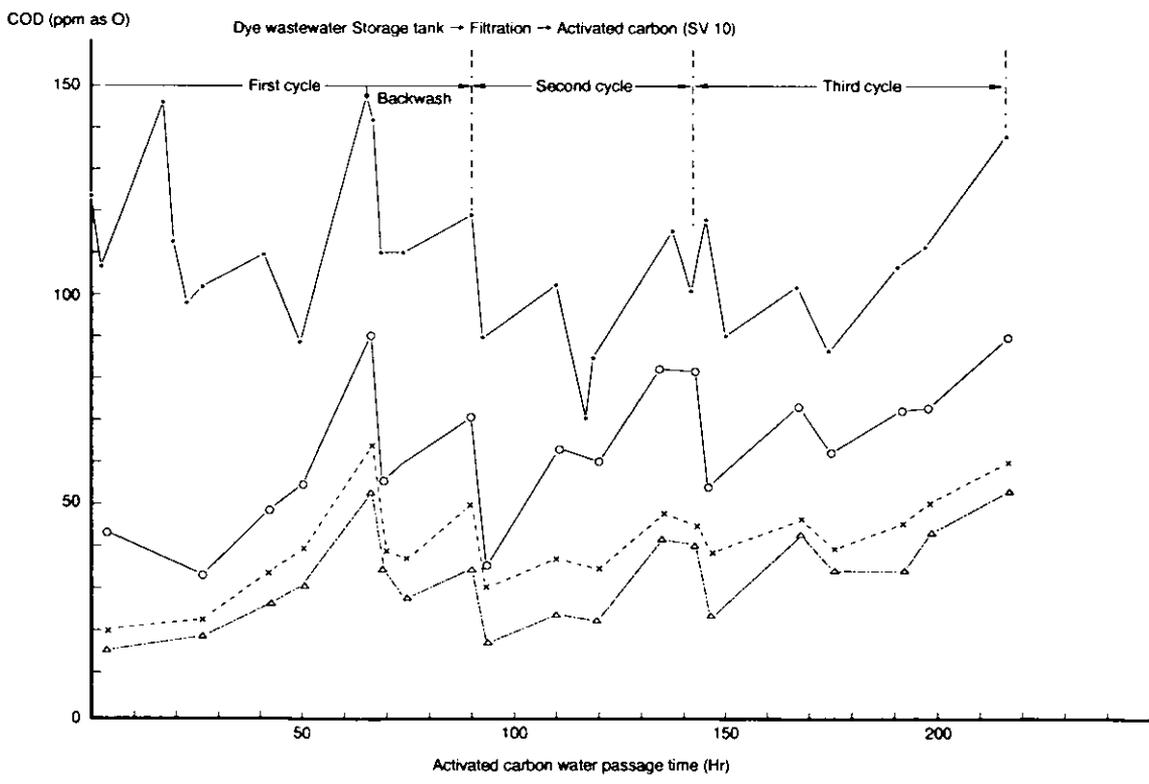
Figure-9 Result of experiment on dye raw wastewater activated carbon adsorption
