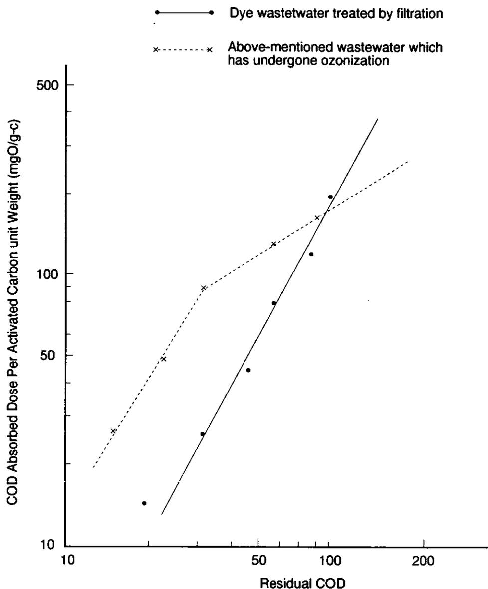
Figure-10 Activated Cabon Equilibrium Adsorption Diagram for Dye Wastewater
