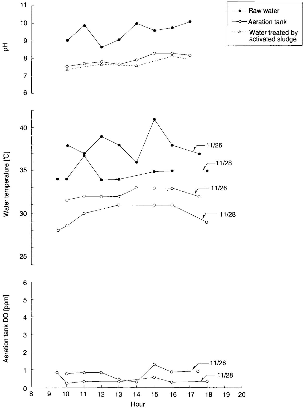
Appended figure-5 Hourly variation in aeration tank DO, water temperature and pH (RUN 4)
