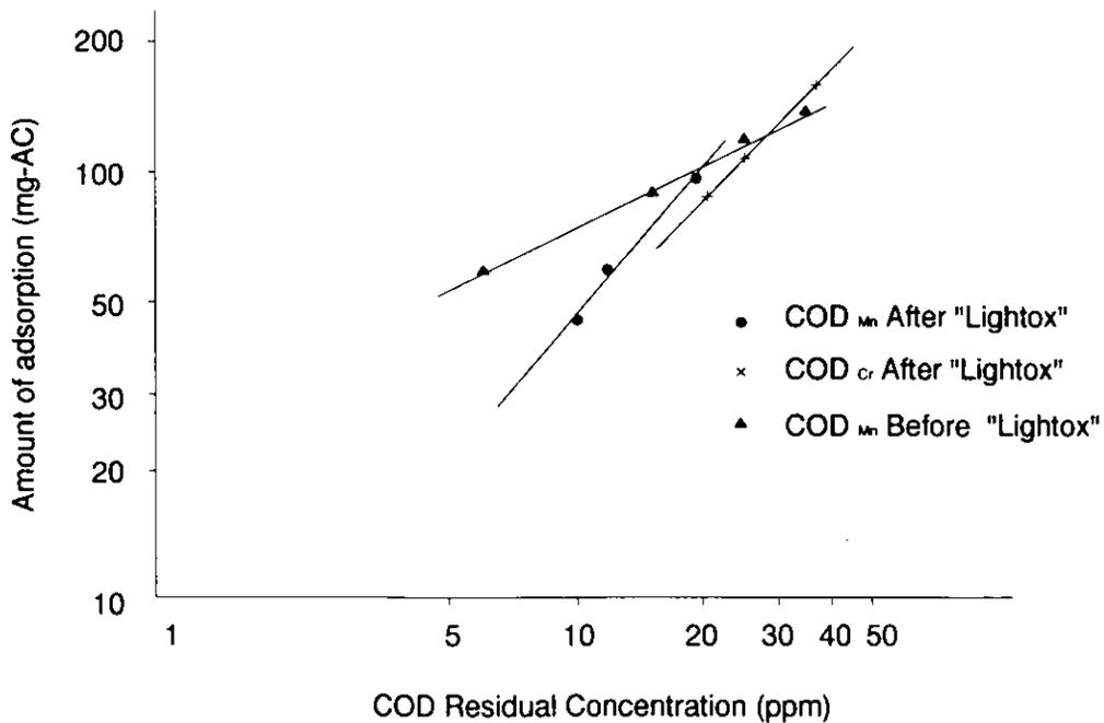
Figure-10 Activated Carbon Adsorption Isotherm
