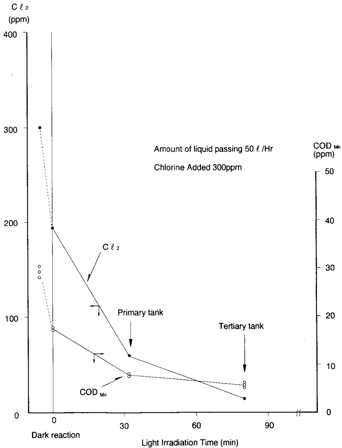
Figure-8 Continuous Test Result (Nov 29. mixing of sulphur dye wastewater)
