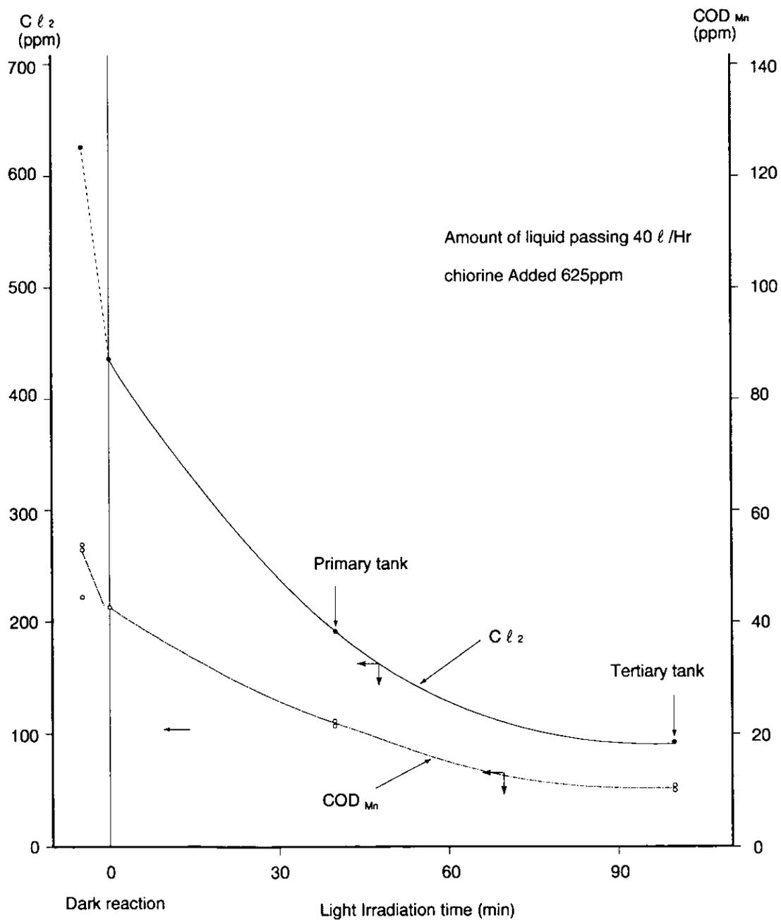
Figure-6 Continuous Test Result (Wastewater of Oct. 28)
