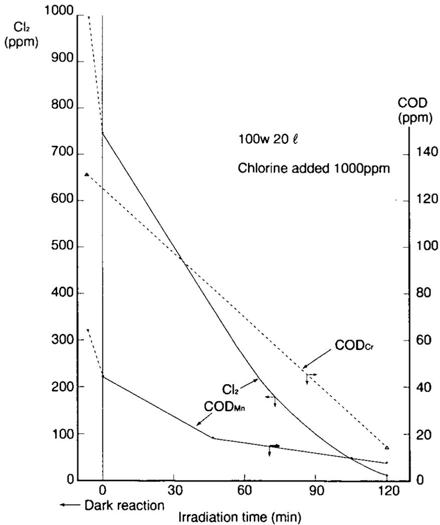
Figure-4 Batch type test result (wastewater of Oct.17)
