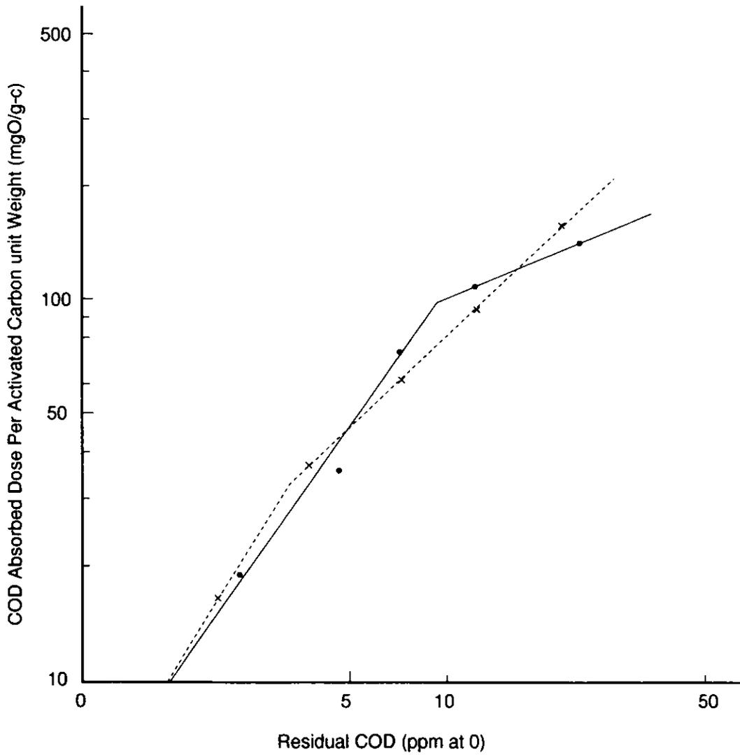
Figure-11 Secondary treatemt water of synthetic wastewater and activated carbon equilibrium adsorption Diagram for its water treated by ozone
