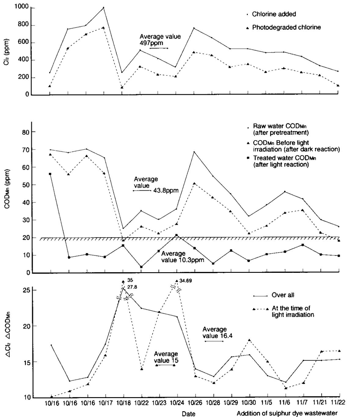
Figure-2 Relation among Quantity of Chlorine, Change in COD<sub>Mn</sub> and  $\Delta Cl_2/\Delta COD_{Mn}$
