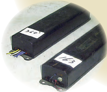
■ Fluorescent Light Ballasts (FLBs) which contain PCB
